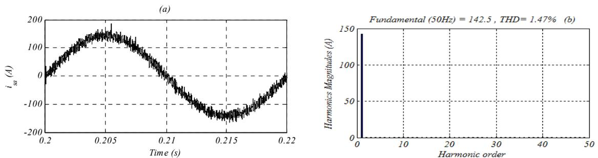
Figure 5. (a) Supply current after harmonics compensation using backstepping controller, (b) Its harmonic spectrum
