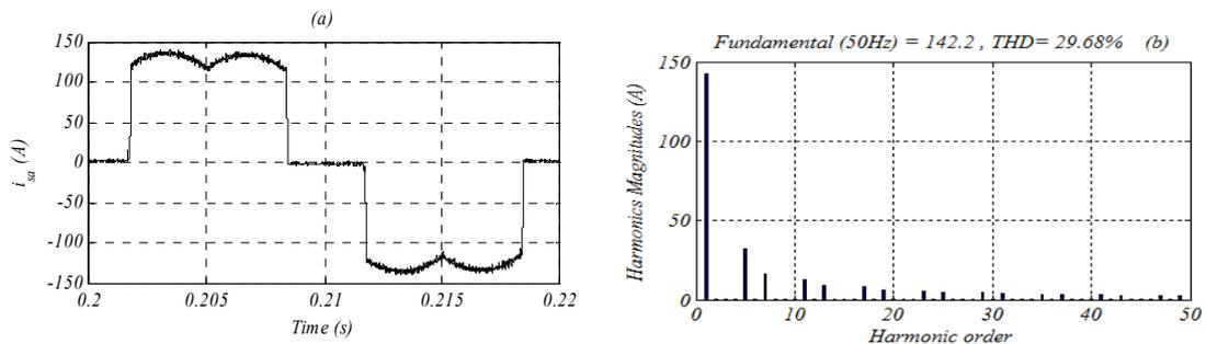
Figure 4. (a) Supply current before harmonics compensation, (b) Its harmonic spectrum
