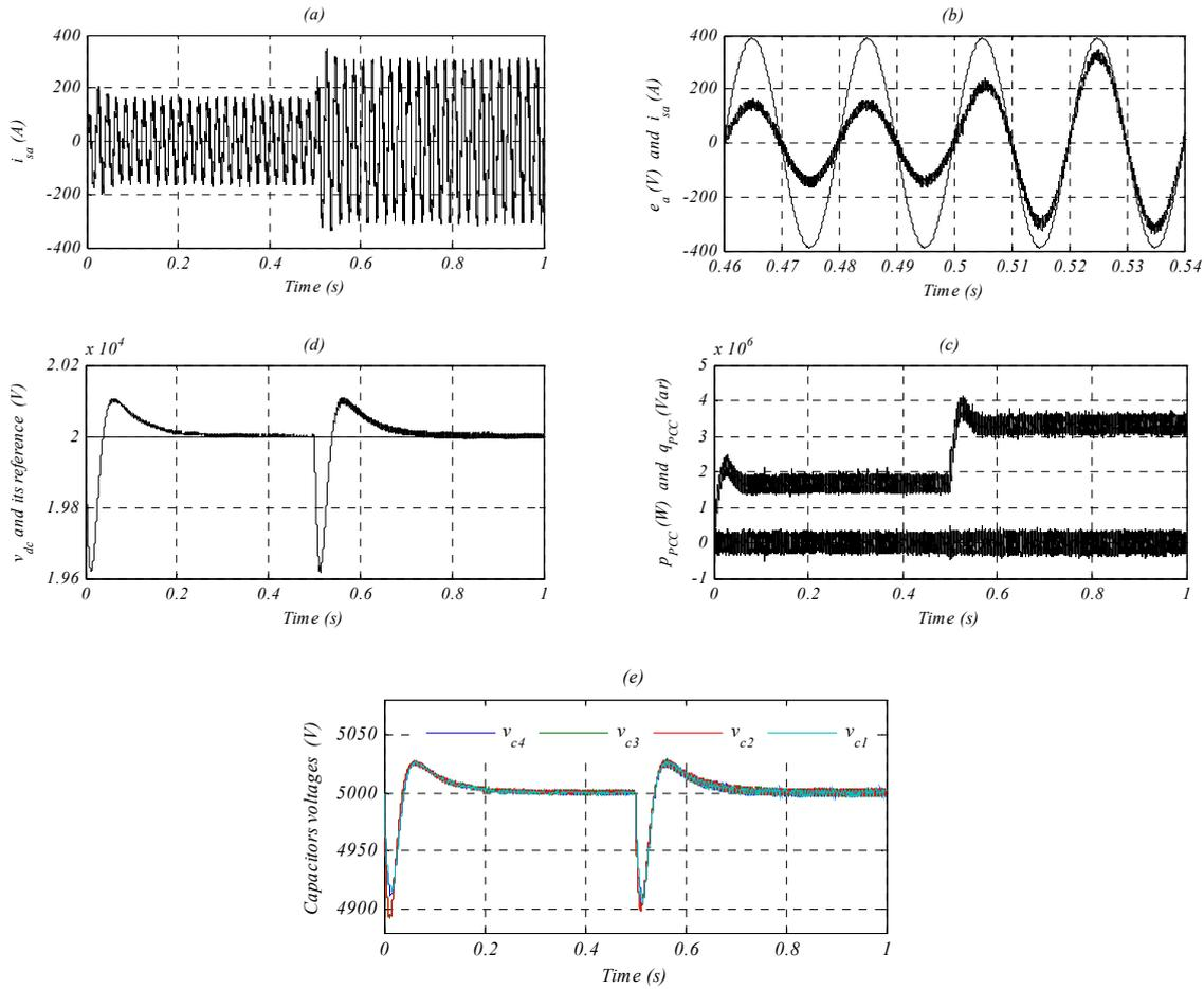
Figure 8. Simulation results of conventional VFDPC-SVM using PI controller. (a) Source current. (b) Reduced source voltage and source current of a-phase (c) PCC active and reactive powers. (d) DC-link voltage  $v_{dc}$ . (e) DC capacitors voltages
