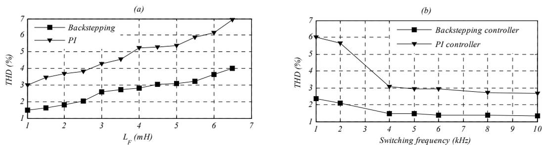
Figure 9. Simulation results of robustness examination. (a) THD of line current versus value of SAPF inductor (b) THD of line current versus value of switching frequency.
