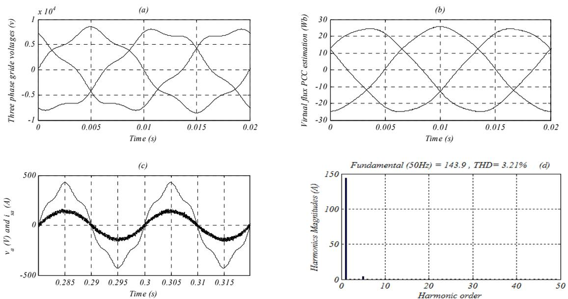
Figure 10. Simulation results of proposed backstepping VFDPC-SVM control with distorted grid phase voltage. (a) Three-phase grid voltages. (b) PCC virtual flux. (c) Reduce source voltage and source current of a-phase. (d) Harmonic spectrum of line current.
