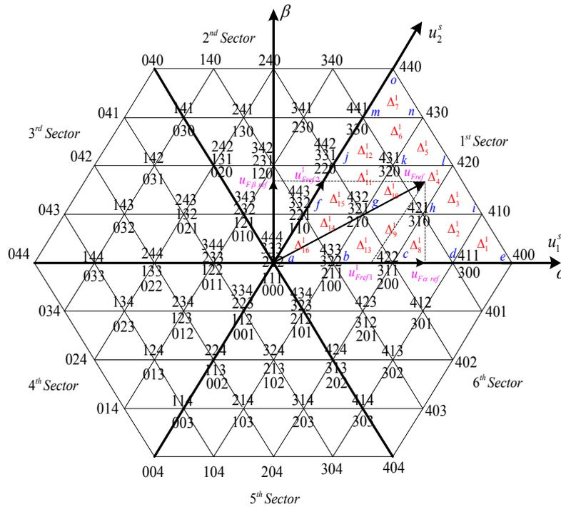
Figure 3. Space voltage vectors for a five-level inverter
