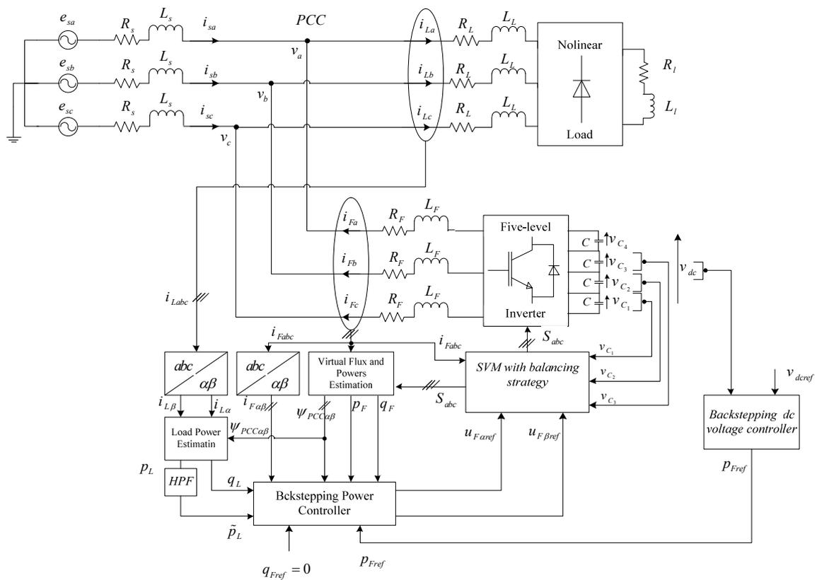
Figure 2. Backstepping VFDP-C-SVM scheme of five-level SAPF
