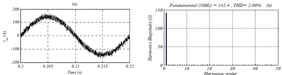
Figure 6. (a) Supply current after harmonics compensation using PI controller, (b) Its harmonic spectrum
