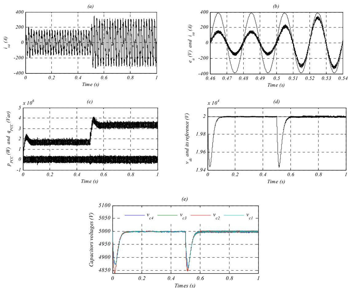
Figure 7. Simulation results of the proposed VFDP-C-SVM using backstepping controller. (a) Source current. (b) Reduced source voltage and source current of a-phase (c) PCC active and reactive powers. (d) DC-link voltage  $v_{dc}$ . (e) DC capacitors voltages
